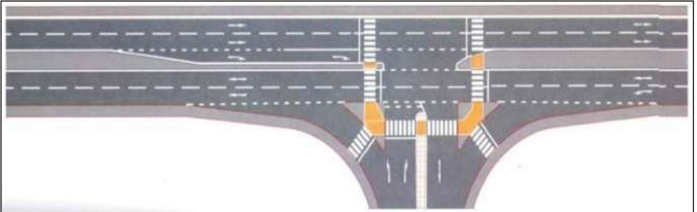
Figure 101: Pedestrian crossing marking on priority junction
