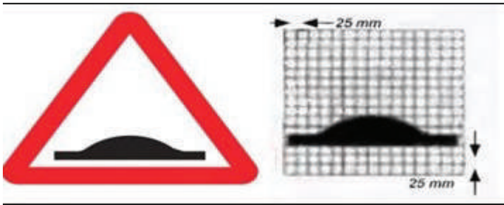
Figure 89: "Speed Breaker" sign
