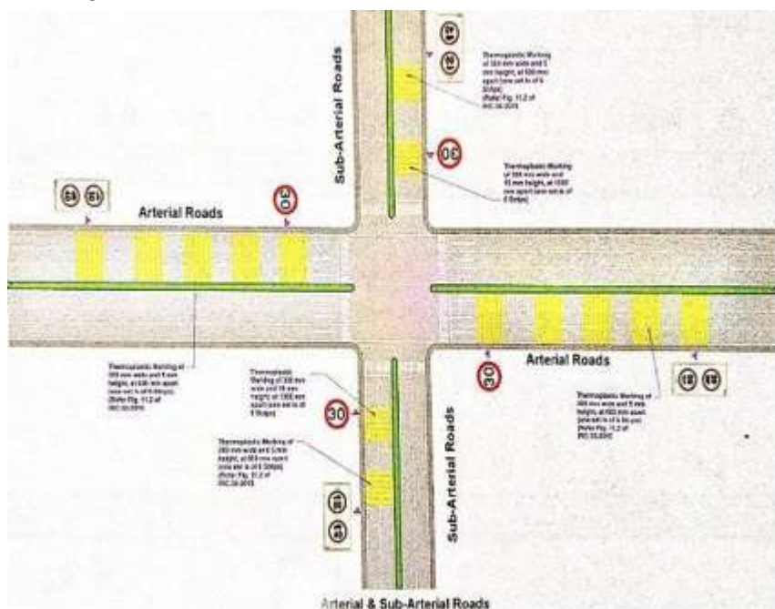
Figure 82: Urban road with traffic calming measures
